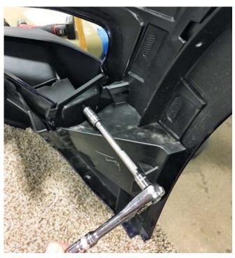
16. Apply one (1) 45° angled washer (1318-12896) onto the corner pocket post as shown. Tighten one (1) nut (PN: W704521). Press the front surface of the corner pocket to the fascia and tighten the nut until snug. Repeat on the other side of the fascia.
