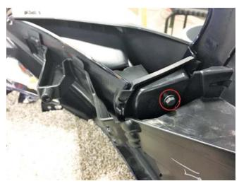
14. Reach under the corner pocket and peel back the double-sided tape red backing. Compress the corner pocket lower edge firmly against the fascia to adhere tape. Repeat on the other side of the fascia.
