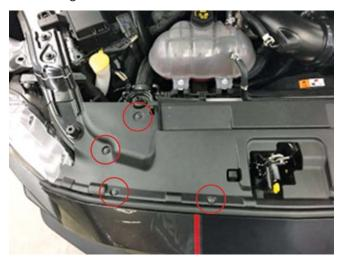
Remove the two (2) 7 mm screws and six (6) 8 mm screws from the upper lip of the fascia. Lift the fascia off the alignment pins and forward off the vehicle (this step may require assistance from another person).
