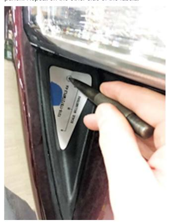
2. Mark the hole center with a punch and drill a 1/8" pilot hole. Drill a 1/4" hole. (**NOTE:** The center of the hole lines up well with the center of the honey comb.) Repeat on the other side of the fascia.
