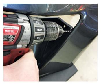
5. Mill out the remaining material in the first, second, and third slots with a dremel or cylindrical file. Repeat on the other side of the fascia.
