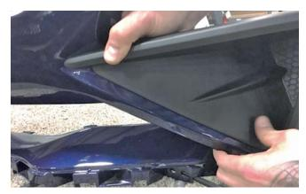
13. Hand start the M5 bolt (PN: 9809A316) to the back of the bracket. Repeat on the other side of the fascia.
