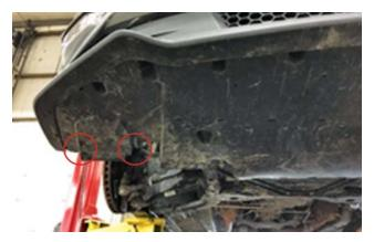
Remove the seventeen (17) (nineteen [19] for performance package) 8 mm screws from the undertray. Remove the two (2) push pins and remove undertray from the vehicle.
