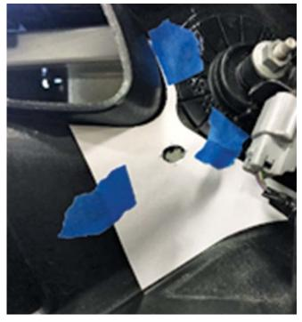
7. Mark the drill hole with a center punch and drill first with an 1/8" pilot hole followed by a 3/8" hole. Repeat on the other side of the fascia.
