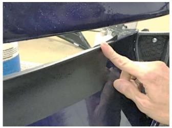
12. Wipe down the surface with isopropyl alcohol. Align the front locator with the forward hole in the fascia and three (3) vertical taps on corner pockets with three (3) slots on the side of the fascia. Repeat on the other side of the fascia. Make sure the flag on the tape is accessible for removal.
