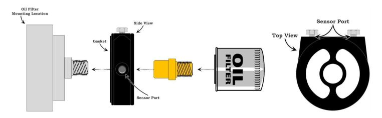
Note: This oil filter sandwich adapter is ONLY for spin on oil filters with a max gasket diameter of 3 inches.
