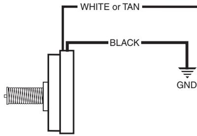
**NOTE:** Never apply power to 2-wire speed sender
